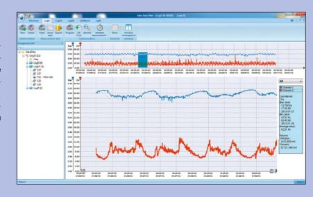
Data set of multiple days showing flow and pressure
