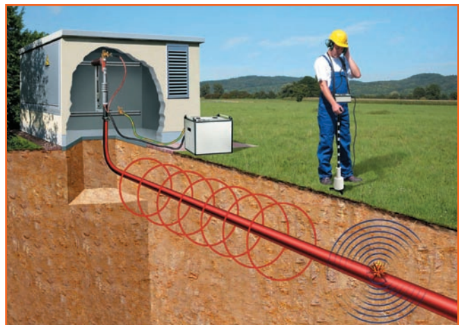
Fault location with SWG and Digiphone
